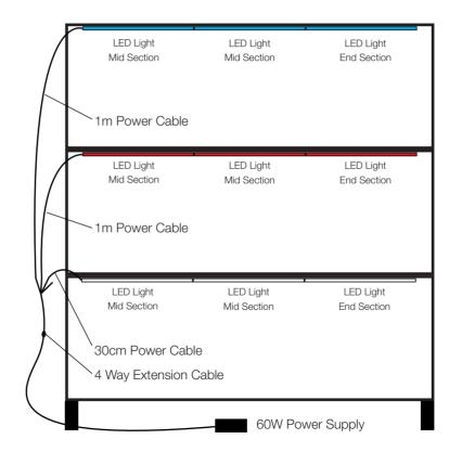
In this example we see a stack of 3 terrariums all lit up from a single power source. This saves on socket space and limits messy wires. Notice, there are 9 light strips in this terrarium stack, so a 60W power supply is required.
